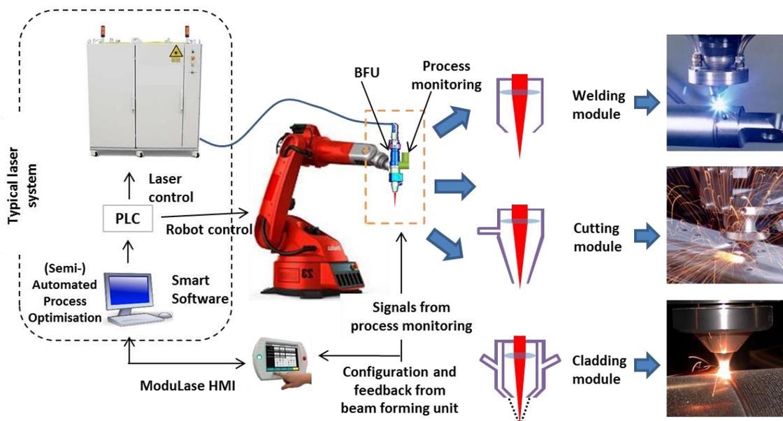
Figure 1 Schematic overview of the ModuLase system, composing a re-configurable process head (with BFU and modular end-effectors), process monitoring sensors, and a control system for adaptive process control and (semi) automated process optimisation.
